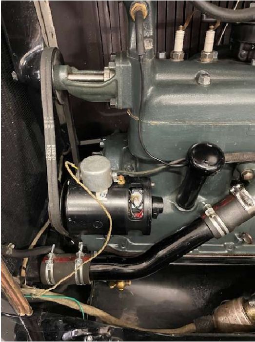
Generator with EVR Installed
