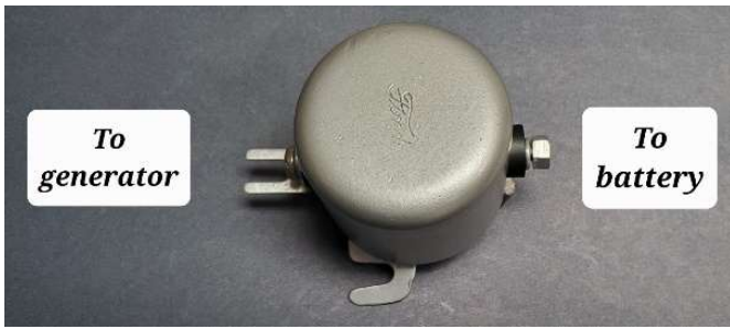
Generator Cutout Orientation
